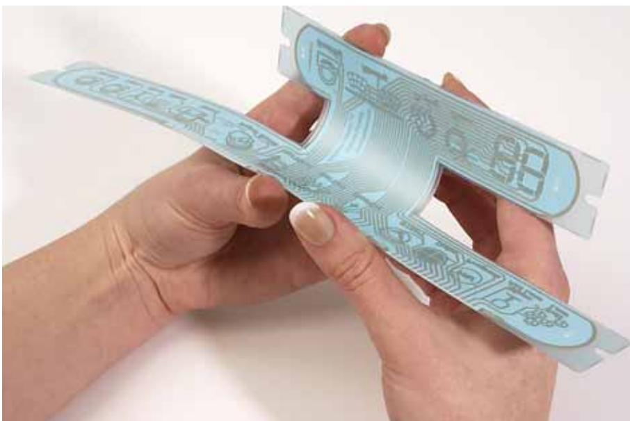
The Pelikon Intuitive Touch Display, a printed flexible electroluminescent display panel
